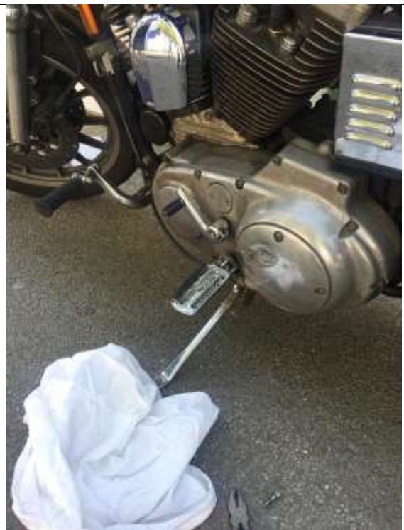
The gear lever before it was repositioned slightly lower to make it easier to use.
